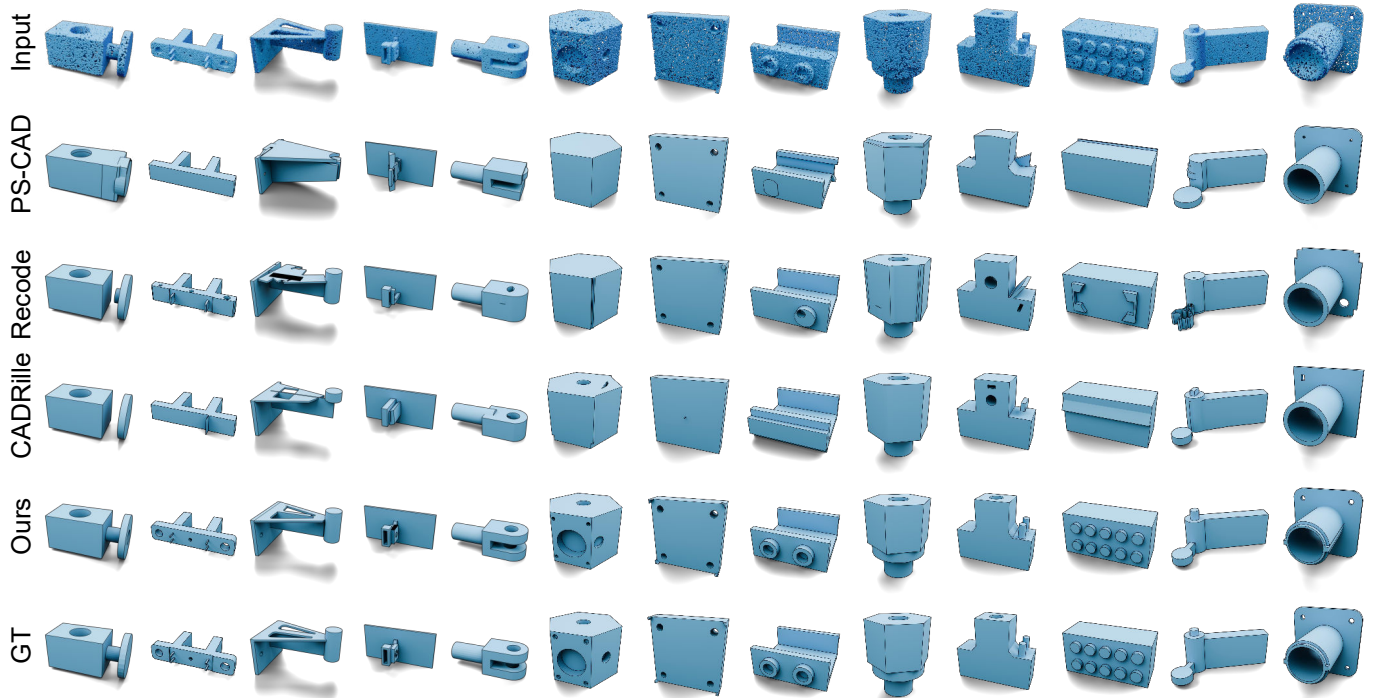
Fig. 8. Qualitative comparison of different methods on DeepCAD. PS-CAD is trained using the DeepCAD training set, while the other methods are trained using CAD-Recode. Please zoom in to see the deviations from ground truth.
